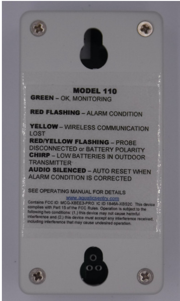
FIG 7 Indoor Alarm Display Rear Cover Operating Instructions
