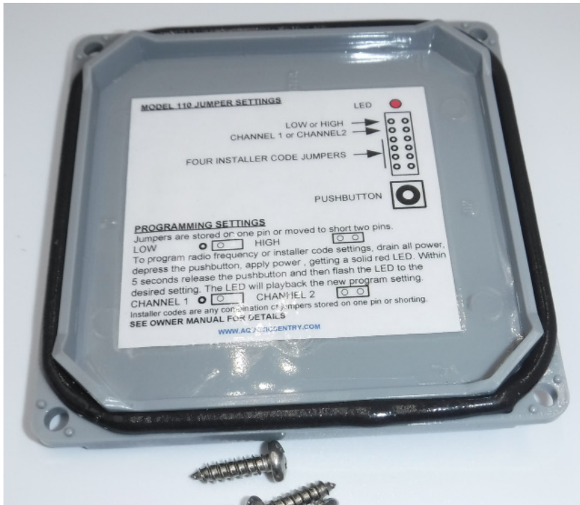
FIG 2 Outdoor Transmitter Enclosure Cover Interior
