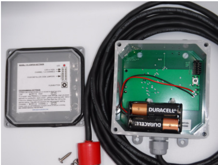
FIG 4 Outdoor Transmitter Batteries Installed
